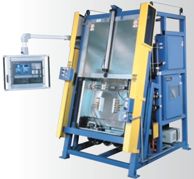
This USAS Leak Test System from VIC Leak Detection tests natural gas meters for American Meter Company
