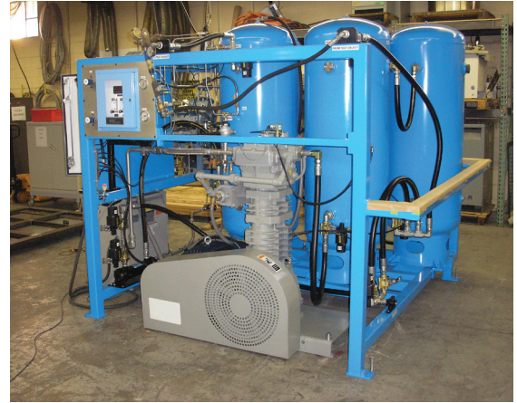
Figure 1. Helium recovery system (Pictured is the VIC Leak Detection 4 SCFM system)
